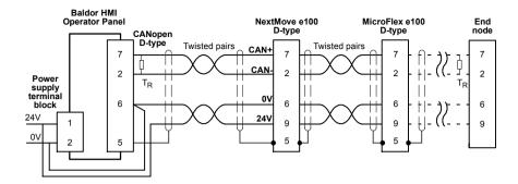
Figure 38 - Typical CANopen network connections
